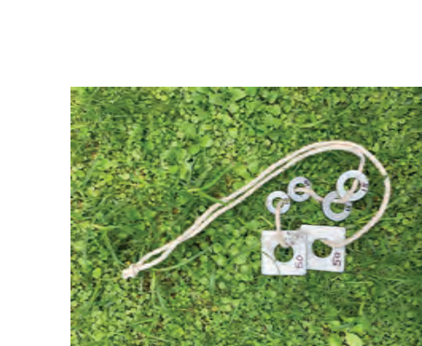
Trap trigger test weights (50g - 150gm)
